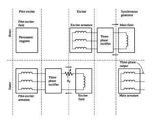
A brushless excitation scheme that includes a pilot exciter. The permanent magnets of the pilot exciter produce the field current of the exciter. Which in turn produces the field current of the main machine.
