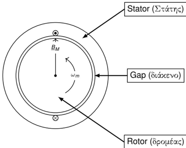
The magnetic field generated by the rotor  $B_M$  is seen by the stator winding as a varying field given by  $B = B_M \cos(\omega t)$ .
