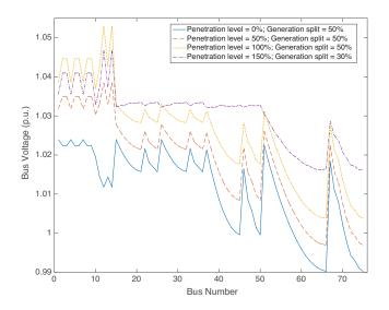
Figure 8. Voltage profile of DN for high penetration levels [Constant load='false', Large system='true', Run OPF='false']
