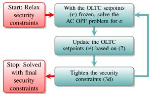
Figure 5. Iterative relaxation technique for the OPF solution
