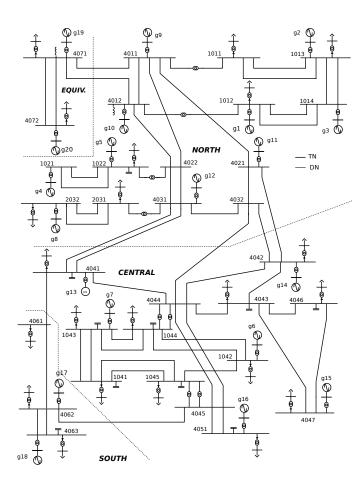
Figure 1. One-line diagram of the transmission network [17]
