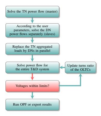
Figure 3. Master-slave approach for the power flow solution
