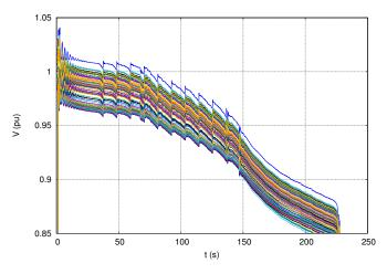
Figure 11. Voltages at various DN buses within the same DN during the dynamic simulation
