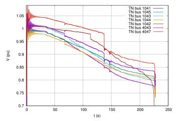
Figure 10. Voltages at various TN buses during the dynamic simulation
