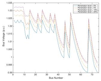
Figure 7. Voltage profile of DN for low penetration levels [Constant load='false', Large system='true', Run OPF='false']
