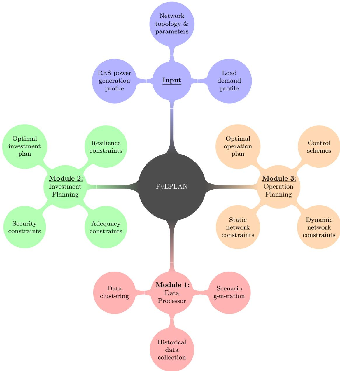
Figure 2.1: Overview of PyEPLAN architecture.
