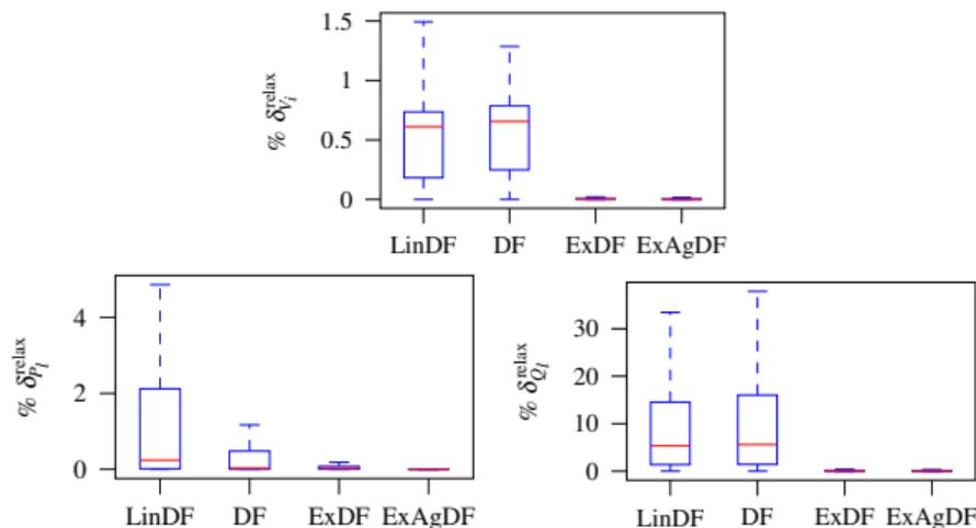
**Figure 2:** Voltage, active and reactive power flow deviations of the different relaxations to the local solution of the NLP model.
