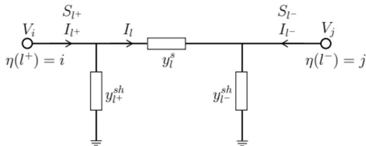
**Model 1:** Extended AC Optimal Power Flow Model (with line shunts)
