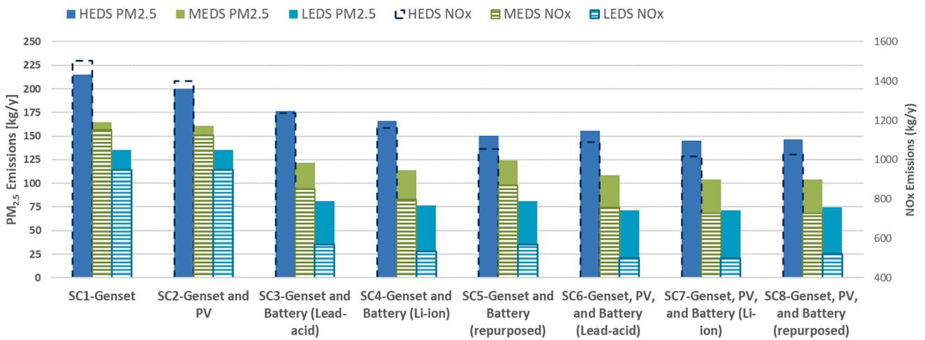
Fig. 8. PM<sub>2.5</sub> and NOx emissions per year for different MG configurations with different load profiles.
