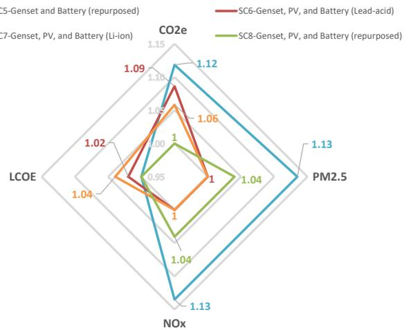
Fig. 13. Pollutant emissions and LCOE comparison for selected LED scenario hybrid system configurations. SC6 and SC7 have the lowest NO<sub>x</sub> and PM<sub>2.5</sub> emissions. SC8 has the lowest CO<sub>2</sub>e emissions. SC5 and SC8 have the lowest LCOE.
